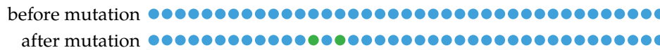
Figure 9.10. Mutation for binary string chromosomes gives each bit a small probability of flipping.
